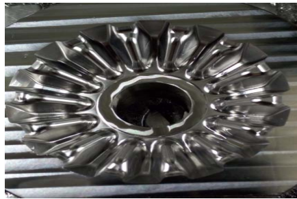
Gear mould: has deep and steep surface, shows the climbing ability and front & back reaction time while machining
