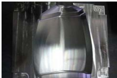
Blowing mould : show the perfect connecting between deep slot curve surface and side wall, also shows the precise & smooth transition of the tool path
