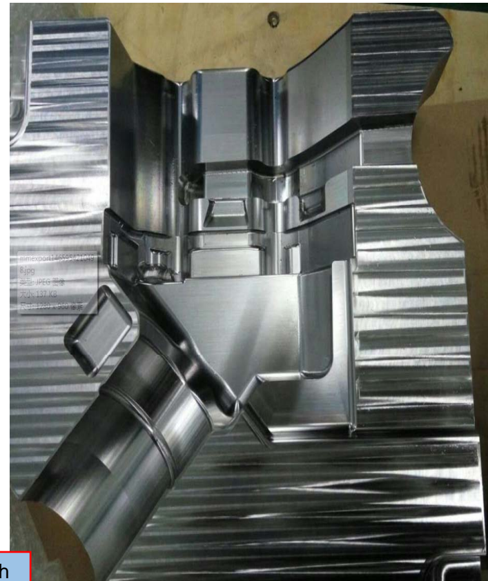
压铸Die casting mould: larger mould will use larger tool to machine. The feeding speed can be increased while the spindle rotate speed is not too high, the mirror like effect can be achieved this way.
