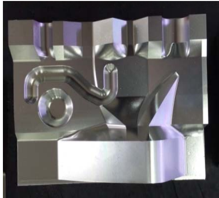
Benz testing part : Inspect the all kinds of accuracy indication and dynamic precision
