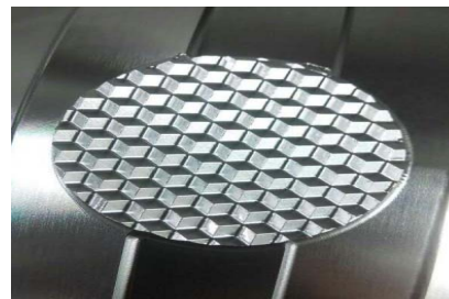
Car's light cover mould: the tool path goes up & down also turns continuously within few millimeters of range, the tool diameter is 0.5 can ensure the surface smoothness, the rotate speed of the spindle can reach 20000rpm
