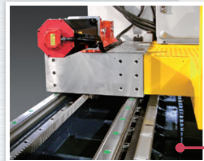
Rack-pinion used on X travel and Y travel SD-48 and up
