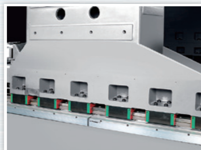
Column & Slider one piece casting
